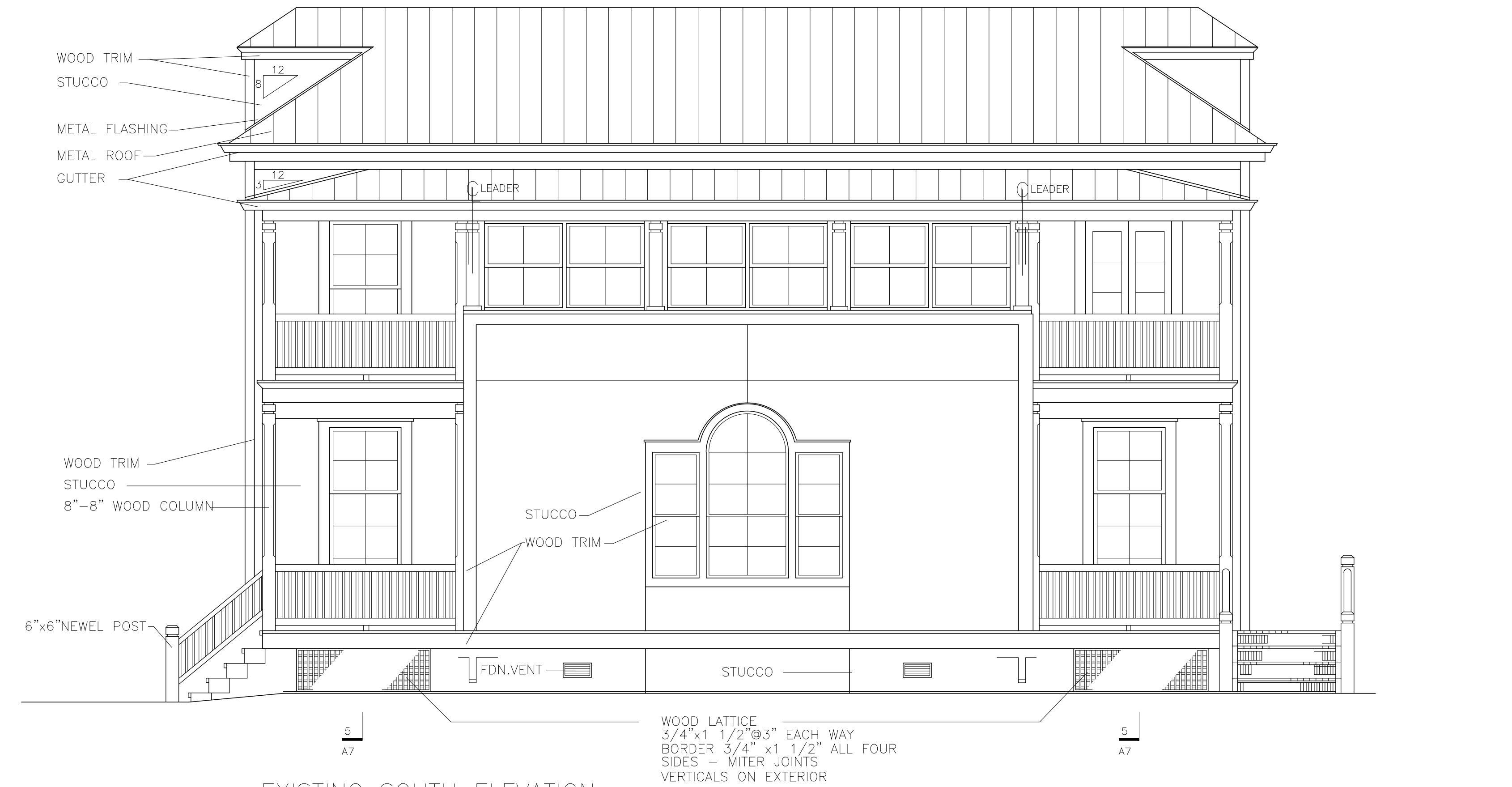
EXISTING SOUTH ELEVATION 1/4"=1'-0"
